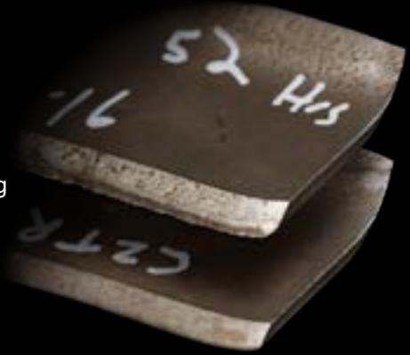
Cutting edge on a standard used blade
