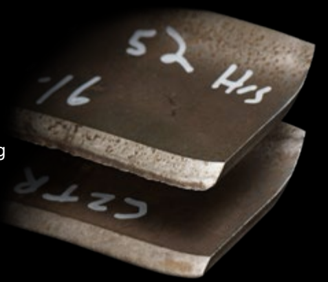
Cutting edge on a standard used blade
