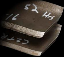
Cutting edge on a used LaserEdge blade
