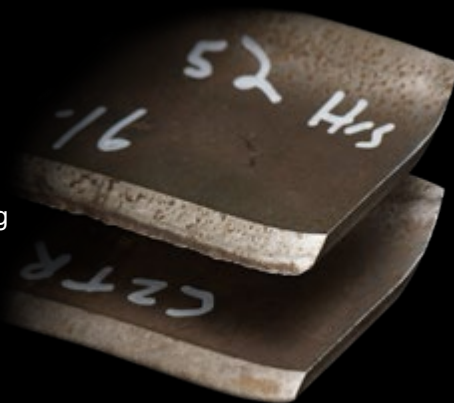
Cutting edge on a standard used blade
