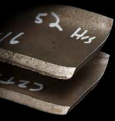
Cutting edge on a standard used blade
