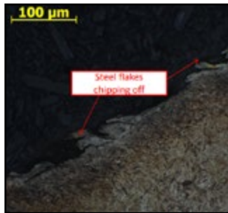
Corrosive Wear viewed under a SEM microscope
