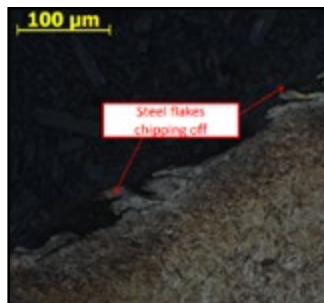
Corrosive Wear viewed under a SEM microscope
