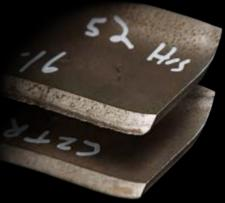
Cutting edge on a used LaserEdge blade
